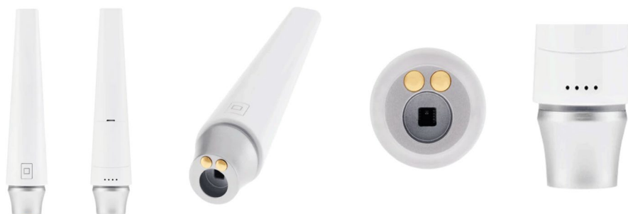
FIGURE 1 Illustrations of the GPSkin probe from different views. The two yellow circles represent the surface hydration sensors; the black square is the RH% sensor located at the bottom of the chamber
